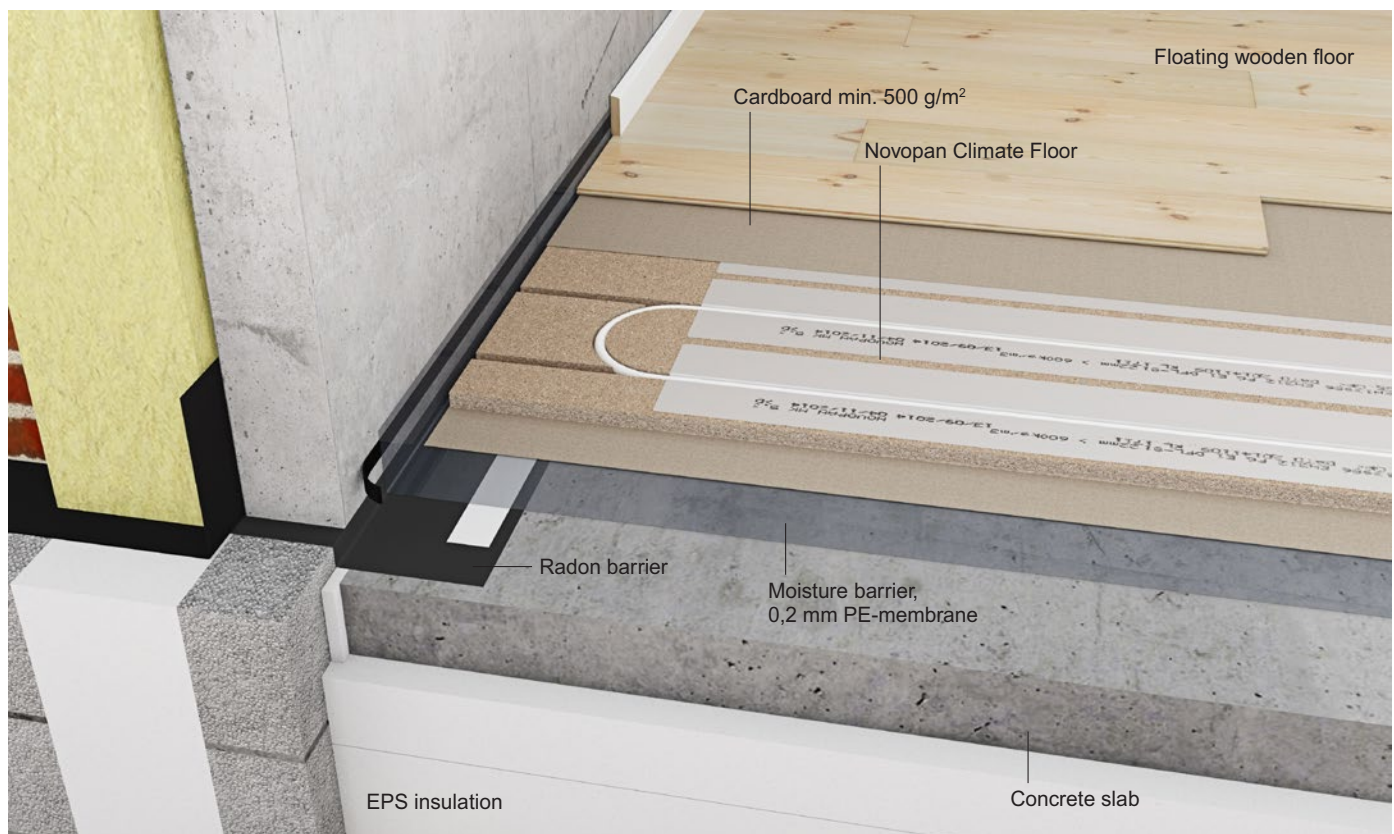
Figure 1 Novopan Climate Floor laid floating on the ground deck and finished with a floating wooden floor.
