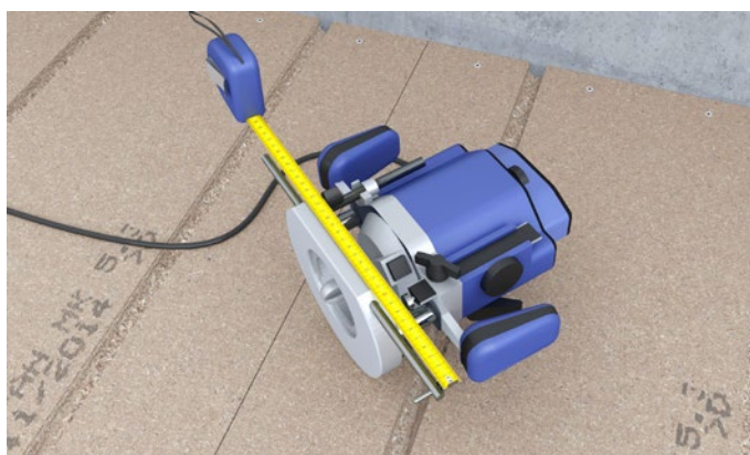
Figure 3 Cutting is carried out with a profile guide to ensure a correct soft turn. The profile guide is mounted in the router land. The distance c-c from pencil screw to router bit is adjusted for use on 22 mm, 25 mm or 38 mm floorboards, see table 1.
