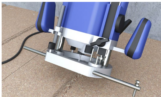
Figure 4 Router bit and cutter depth are selected and adjusted, see table 1. Pencil screw may be adjusted in height and countersunk.
