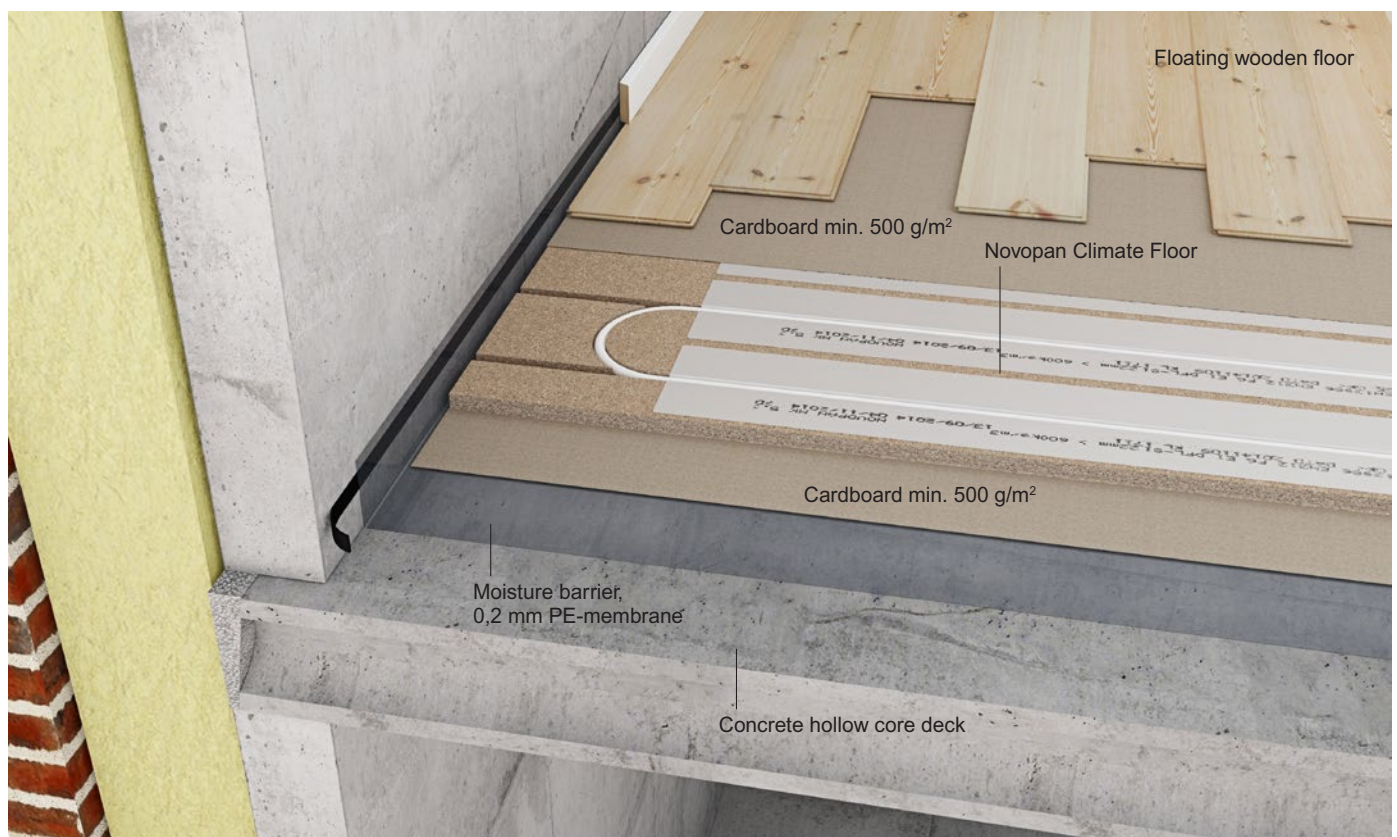
Figure 1 Novopan Climate Floor laid floating on a concrete floor deck and finished with a floating wooden floor.
