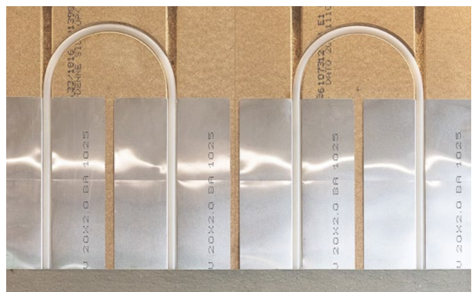
Figure 3 Heat emission plates for 16 mm heating pipes, groove spacing 200 mm cc.
